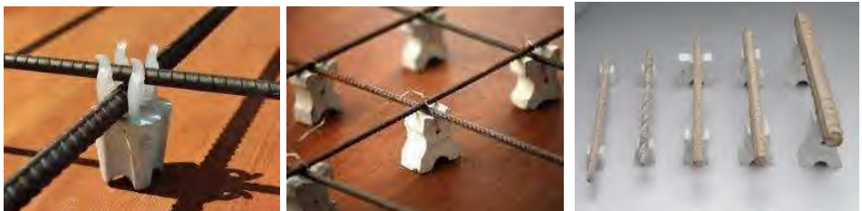
Figure: A Cover Block is essentially a spacer that is used to lift the rebar matrix off the ground so that concrete may flow underneath the rebar.
