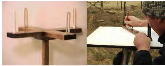
Figure: A sighting device or pointer for determining directions or measuring angles, used mainly in surveying.
