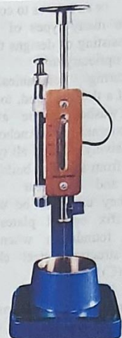
Figure: Vicat's apparatus for determining consistency of cement.
