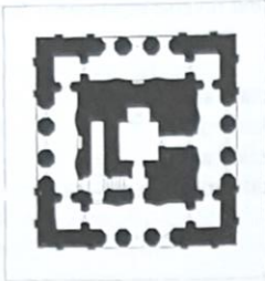
Figure: Plan of Shyam Rai Temple, Bishnupur. This brick-built Temple is situated within the fort and consists of a square roof surmounted by five towers and is thus an example of Panchratna type. The central tower itself is octagonal enclosed by an octagonal corridor. The temple is the most profusely carved temple in Bishnupur. Inscription records erection by Raghunatha Singha in 1643 AD. Source: asikolkata.in/bankura.aspx
