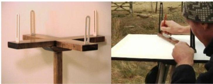
Figure: A sighting device or pointer for determining directions or measuring angles, used mainly in surveying.
