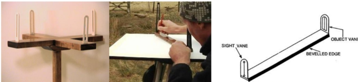
Figure: A sighting device or pointer for determining directions or measuring angles, used mainly in surveying.
