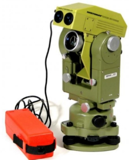
Figure: Distomat is the trade name of E.D.M (Electronic Distance Measurement) manufactured by LEICA Company of Switzerland. This instrument uses infra-red light as signals. It is a very small, compact EDM instrument, particularly useful in building construction and other Civil Engineering works, where distance measurements are less than 500 m. It is an EDM that makes the meaning tape redundant. Through EDM, Direct measurement of distances and their directions can be obtained by using electronic instruments that rely on propagation, reflection and reception of either light waves or radio waves.
