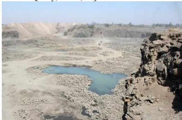
Figure: A 200-acre exhausted basalt quarry in Timba. Basalt deposits were mined up to depth of 20m. Vegetation were in poor condition. Unwanted stones and quarry dust were heaped all over.
